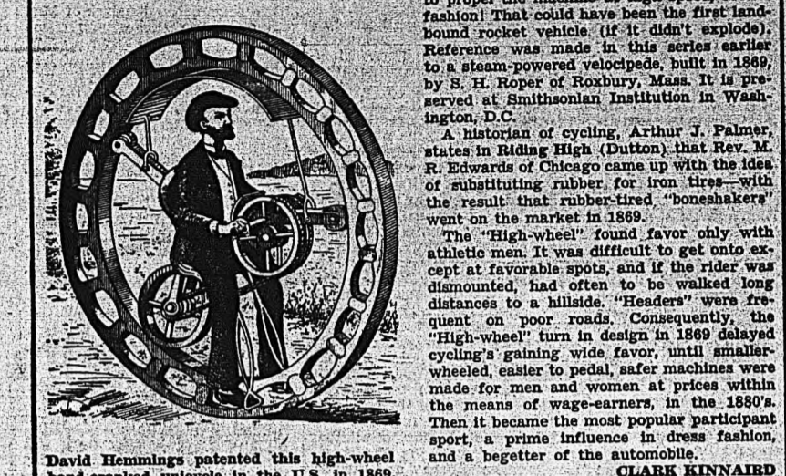
David Hemmings patented this high-wheel hand-cranked unicycle in the U.S. in 1869. CLARK KINNAIRD
