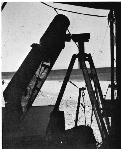
Telescope feeding Fabry-Perot interferometer, used in Prof. Schmitt's experiment on solar corona visible wavelengths.
