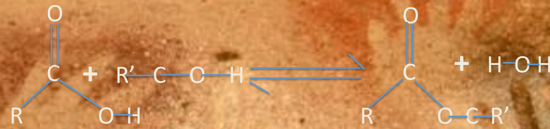
Figure 1: Fatty Acid to Fatty Acid Methyl Ester Process, R and R' are methyl groups
