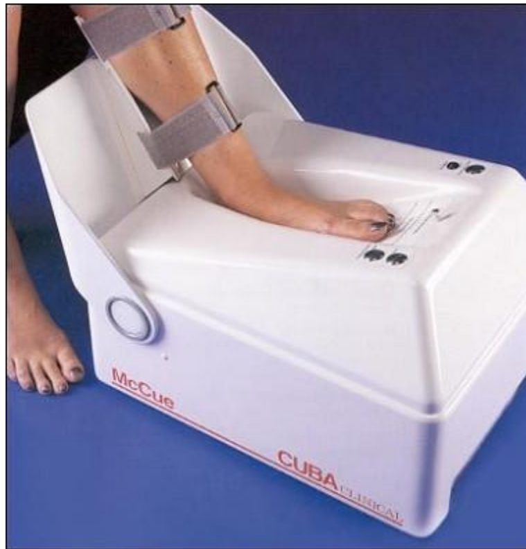
Figure 1.5: A typical ultrasonic measurement system to analyze the density of a heelbone using through-transmitted ultrasound.
