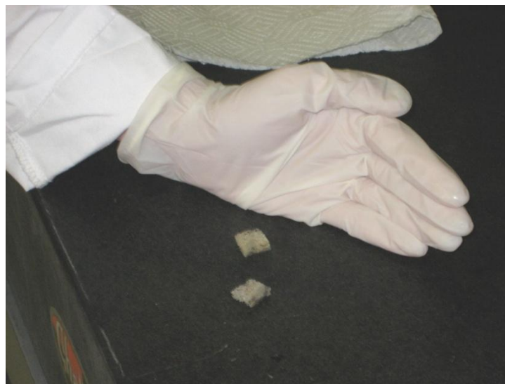
Figure 2.1: Two specimens of cancellous bone in slices approximately 5 mm x 15 mm x 15 mm.
